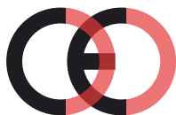
False CE Mark (too close)
